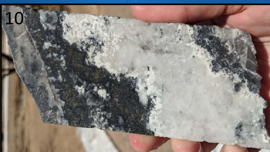
10 2.2m @ 61.36 gpt Au, 2833.5 gpt Ag, or 7436 gpt AgEq including 0.4m @ 305.0 gpt Au, 13889.5 gpt Ag, or 36764 gpt AgEq
